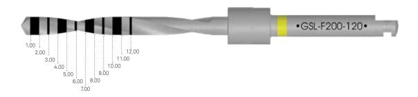
The depth notches, common to all drills, are at a distance of 1 mm between each of them.
